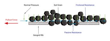
Interaction between the Soil and the Geogrid/Geotextile
